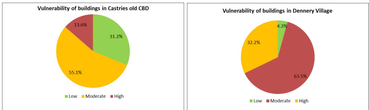
Figure 7-11: Physical vulnerability of buildings in Castries old CBD and Dennery Village
