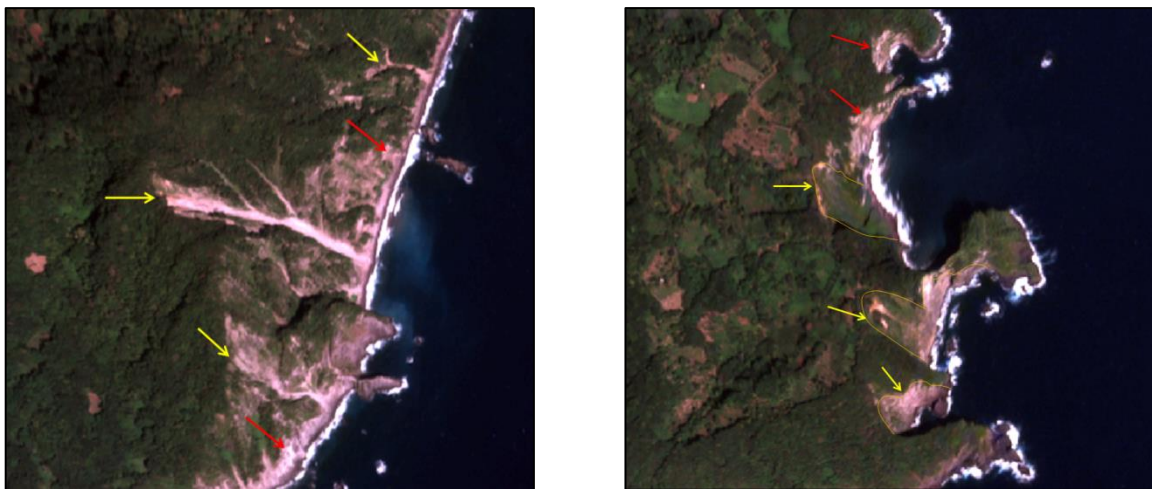
Figure 12. Examples of Landslide image interpretation in Dominica. A. The yellow arrows indicate Debris Slides (Left) and B. Rockslides (Right). The red arrows show areas of Rockfall.
