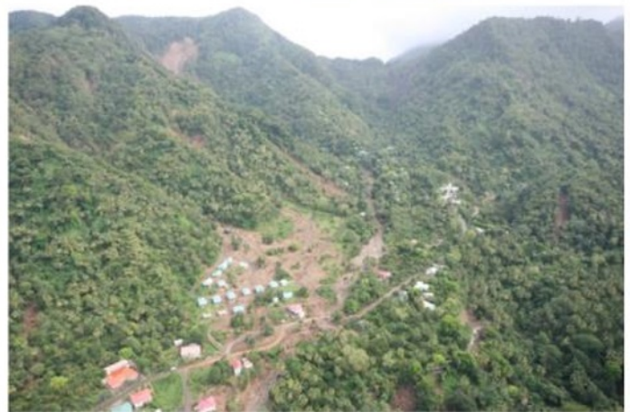
Figure 5: Google Earth image showing the large landslide on the confluence of Mathieu River and Layou River in Dominica that created a dammed lake which broke out catastrophically later.
