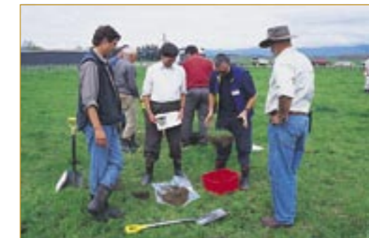
The drop shatter test. The sample is dropped a maximum of three times from a height of 1m (waist height) onto the wooden square in the plastic basin. The soil is then transferred onto the large plastic bag and graded so that the coarsest clods are at one end and the finest aggregates are at the other end.
